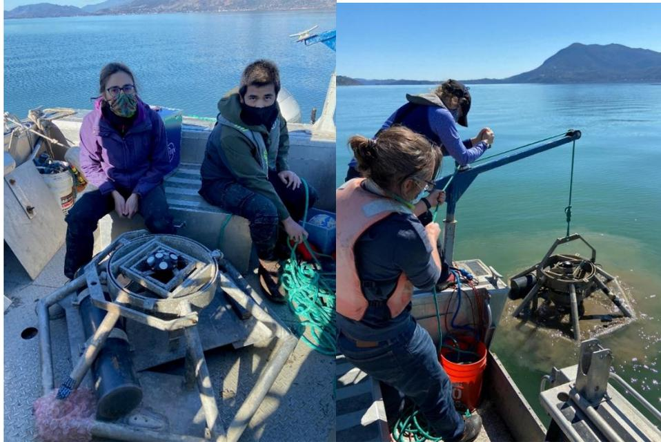
Figure 7.10.1. Field work photos during the deployment of an ADCP at Clear Lake
